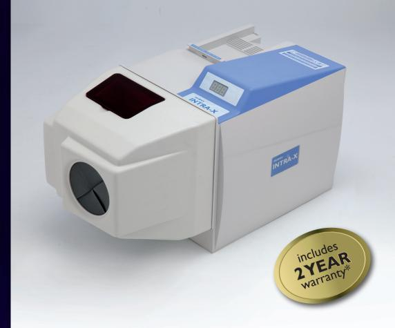
The Velopex Intra-X Processor (Daylight) can process all sizes of Intra-oral dental films from size 0 (22x35mm) to size 4 (57x76mm) Dry-to-Dry In under 5 minutes – endo-interrupt facility (size 2, 30x40mm) allows intra-oral film to be removed (wet) after 2 minutes (after fixer). Unit features: auto-start and digital timer display. It comes with magnetic chemical agitation and a free chemical replenishment system to prolong chemical life.
